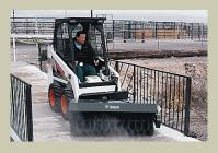
**Angle Broom**Sweeps snow, dirt and debris from driveways, loading docks and warehouse floors.
